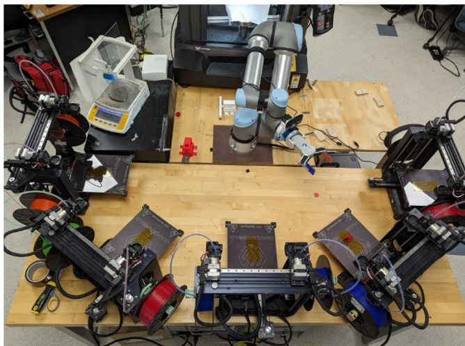
Fig. S5 | Picture of the Bayesian experimental autonomous researcher (BEAR), consisting of five fused filament fabrication 3D printers, a six-axis robot arm, a scale, and a universal testing machine.
