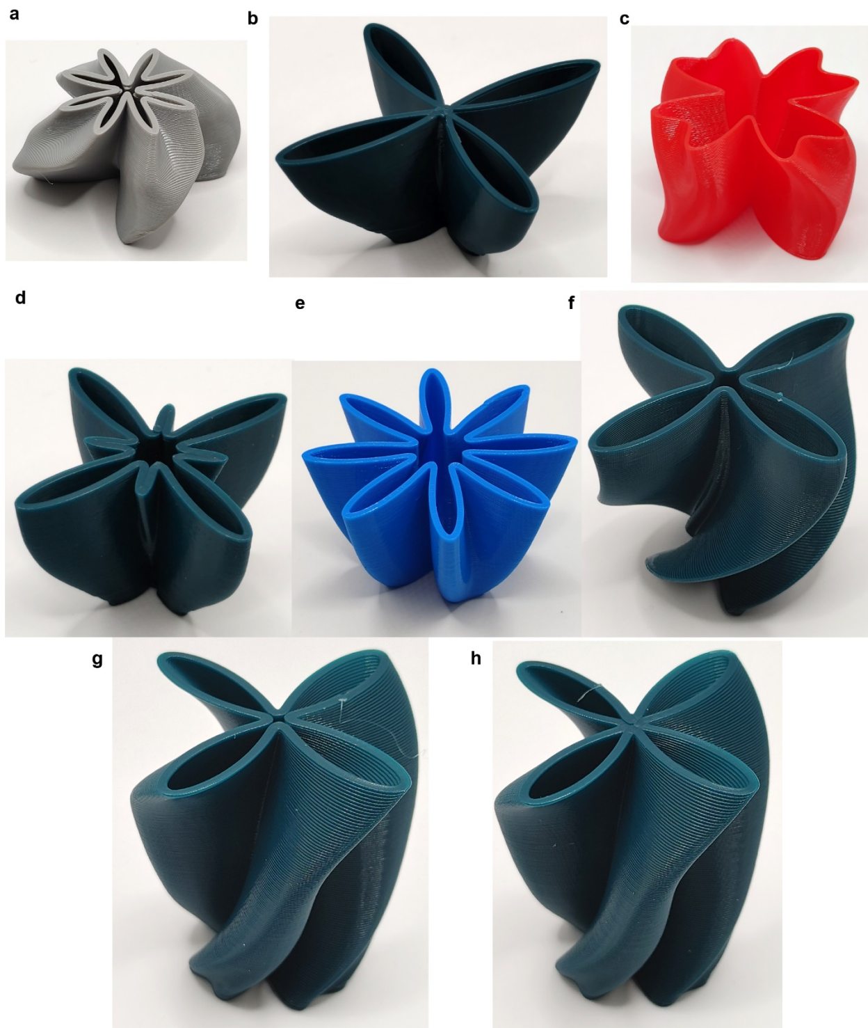
Fig. S11 | Enlarged images of noteworthy components. a-h, Pictures of noteworthy parts that significantly improved K_s^* during the course of the campaign, as seen in Figure 2a. Heights vary from 19 mm (a-d) to 27.8 mm (g). Maximum widths range from 29 mm (g) to 48 mm (b). The color of the pictured components is indicative of the material used, with Green indicating PLA, Blue indicating PETG, Red indicating TPU-2, and Gray indicating TPU-3. Pictures are reprints, as the original parts were deformed during initial testing.
