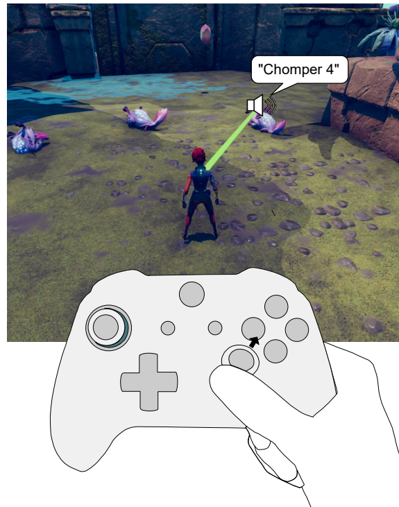
Figure 1: Overview of NavStick. Top: A player looks around for enemy “Chompers” within The Explorer , our prototype 3D adventure game. The green line represents their scrubbing direction; they are scrubbing at one o’clock and will hear the system read “Chomper 4” via spatialized audio. Bottom: A player uses their game controller to look around for enemies using NavStick. Here, the player is pushing the right stick in the one o’clock direction.
